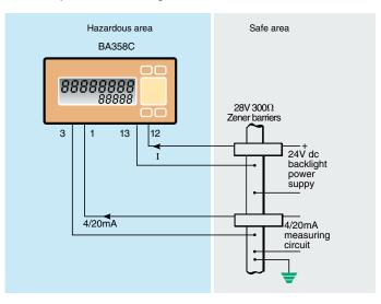
Figure 7 Backlight power supply
