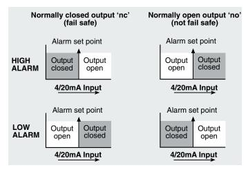
Figure 4 Alarm outputs
