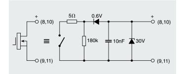
Figure 5 Equivalent circuit of each alarm output
