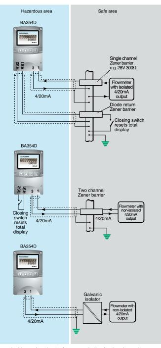
Figure 3 Alternative circuits for remote indication in a hazardous area
