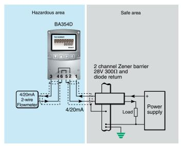
Figure 2 BA354D displaying rate of flow and total flow in hazardous area
