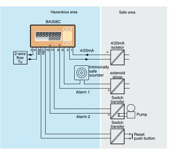
Figure 6 Typical application of BA358C with alarm outputs
